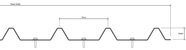
For fixing to steel, Colour-Matched 12-14 x 25mm Hex Washer Face Head Self-Drilling Screws are ideal.
